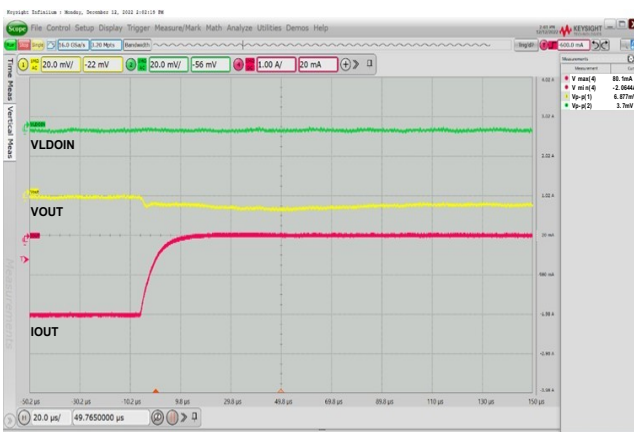
Vout Load transient test : Sinking current Iout from 2A to 0A
